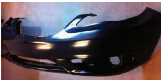
Example of low temperature cured GMA powder coating on automotive bumper
