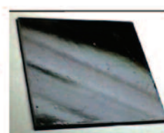
Almatex AP4411 based GMA powder coating contaminates into black polyester powder coating causing no craters
